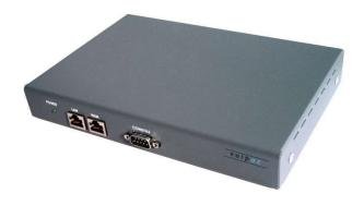
Linux operating system is preinstalled on the board as default. Board is manageable through standard RS232 serial link. For the effective work, user should use terminal station. Later when network interfaces are configured user can manage whole system remotely via LAN/internet using SSH protocol. Also remote software upload/upgrade is supported by system. There can be customer made applications stored in FLASH memory.
