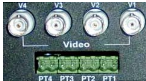
The BNC video input and PT controller connectors
